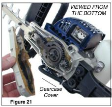
Remove the gearcase cover, and use solvent and a soft brush to remove all old grease from the gearcase. To refill, hand-pack the gearcase with approximately 40–50 grams of high quality lithium-based grease (50–70% of capacity). DO NOT OVERFILL!
